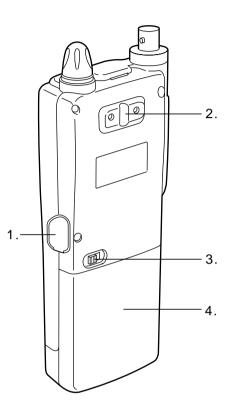
**1. DC-IN** Connect an external DC supply here (10 - 16 V).
