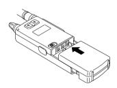
Fit the battery pack into the holes on the DJ-X2000 and push in the direction of the arrow until the case snaps into the place.
