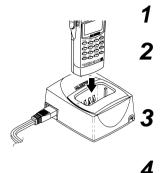
Plug the AC power cord into the AC power socket on the battery charger.
