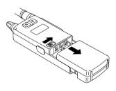
Slide the battery pack lock on the case to the right and pull the case downward to detach.
