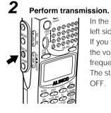
In the TRANCEIVER mode, the O key located on the left side of the DJ-X2000 works as the **PTT** key. If you speak to the microphone when the **PTT** key is ON, the voice can be transmitted at the currently received frequency.
